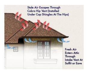
**DO NOT use multiple vent systems:** In general, if continuous soffit or fascia and ridge vents are used; power fans, roof louvers, static exhaust vents and any other roof vents should be removed or disconnected and gable vents should be closed. The use of mixed ventilation systems, such as soffit and ridge vents in combination with a power fan could result in reverse airflow that could result in water leakage into the attic.
